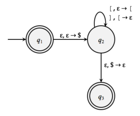
Recall: A transition of the form a, b → z means "if the current input symbol is a and the current stack symbol is b, then follow this transition, pop b, and push the string z"
