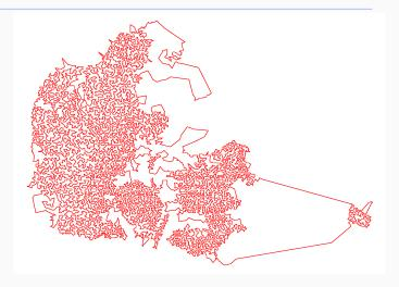
This is an *optimal* solution for a TSP instance with tens of thousands of points; obtained using MIP-like techniques.
