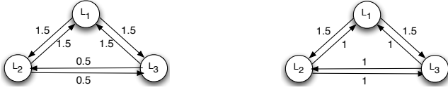
Figure 2: Peers L_1 , L_2 and L_3 with upload capacities 3, 2, and 2. Bandwidth allocated under FairTorrent (left) vs Equal-Split (right).
