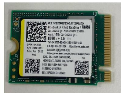
Figure 25: A 256GB NVMe SSD from a Dell laptop. This device is roughly the size of the first digit of your thumb. In 2025, an SSD can store data at a cost of roughly \$0.040 per billion bytes.
