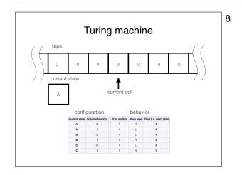
Here is one standard language model: the Turing machine. Its operation is very simple. See if you can determine its next steps using the table below.
