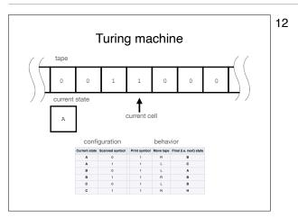
... move the tape to the left and update the current state to A. And so on until the machine halts ("H").
