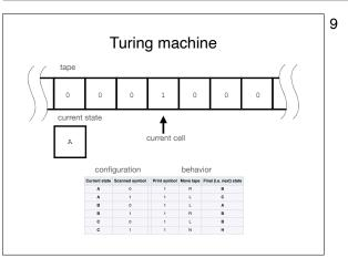
When in state A and current symbol 0, we write a 1 to the tape, then...
