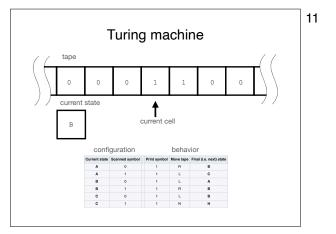
Next, with B in the current state with 0 in the current cell, we write a 1 and ...
